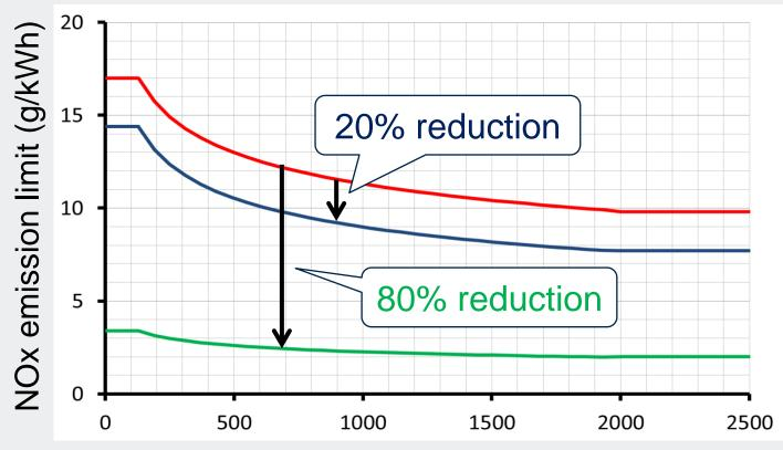
Rated engine speed (rpm)
